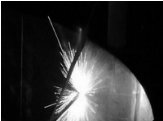
Figure 2 The photo of shunts spark discharge
