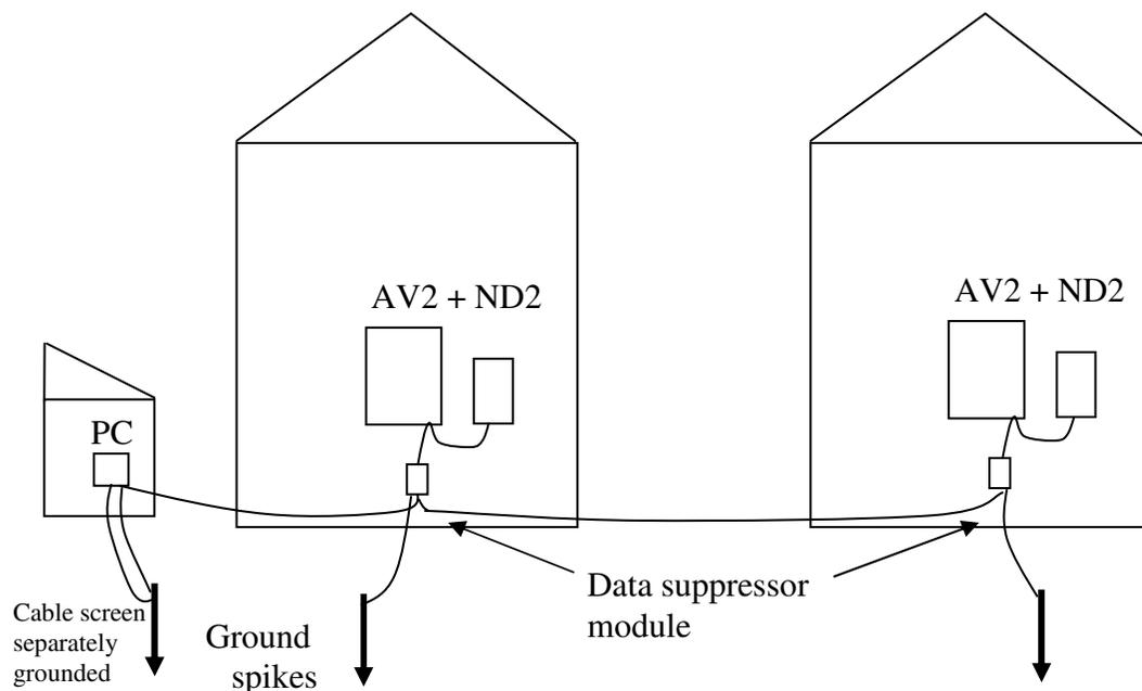
Note that the stub of cable connecting between the suppressor module and the local controller(s) should not exceed 1m to 2m at the most. Also note that the cable screen is grounded separately at a single point in the system, normally at the master device.
