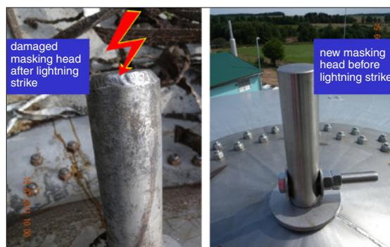
Fig. 4. Comparison of the upper parts of fermenters after and before lightning strike
