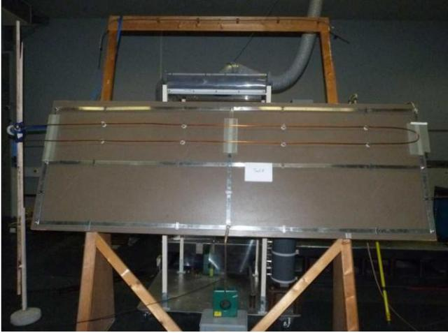
Figure 11. Construction model for measurement with conductive loop placed at the upper position
