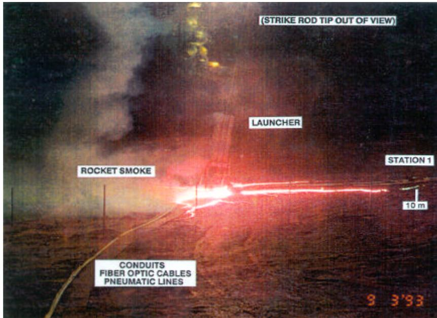
Figure 2. Photograph of the surface arcs emanating from the ground rod conducting a 29.6 kA rocket-triggered lightning strike to ground at Fort McClellan, AL. (Fisher and Schnetzer, 1994)
