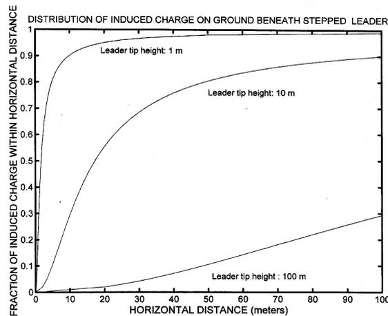
Figure 4. A plot of the distribution of induced charge on a conducting surface beneath a point charge.
